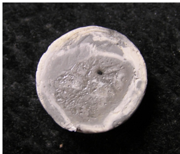
Fig. 8. Photograph of the surface of tin slug in contact with the electrolyte for the button cell sample. The ring of wing around the circumference is SnO_2 .
